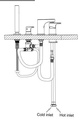
Attach the shower hose (W) to the shower (U) and diverter assembly (Q). Attach the spout assembly (A) and controller (E) to diverter assembly (Q) using braided hoses provided.
